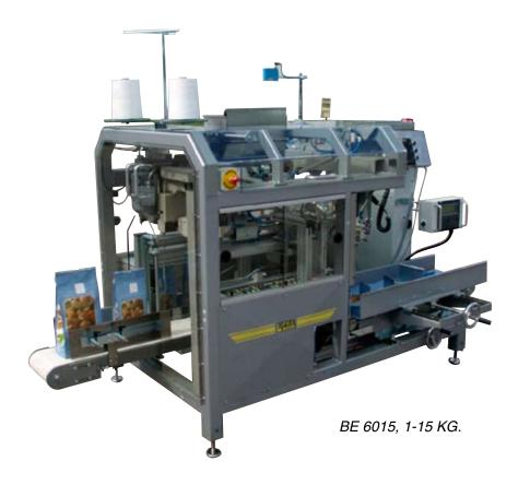
The BE 6015 Papper Bagger is designed for fullautomatic packaging of potatoes, onions or other products in 1-15 kg paper bags either with or without handles. The papper bagger can be connected to electronic scales. The bag magazine will hold approx. 250 bags and can be continously fed. Switching over from one size of bag to another is simply carried out by setting the computer.
