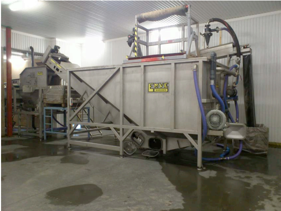
EMVE Soakingtank with Boxturner.
