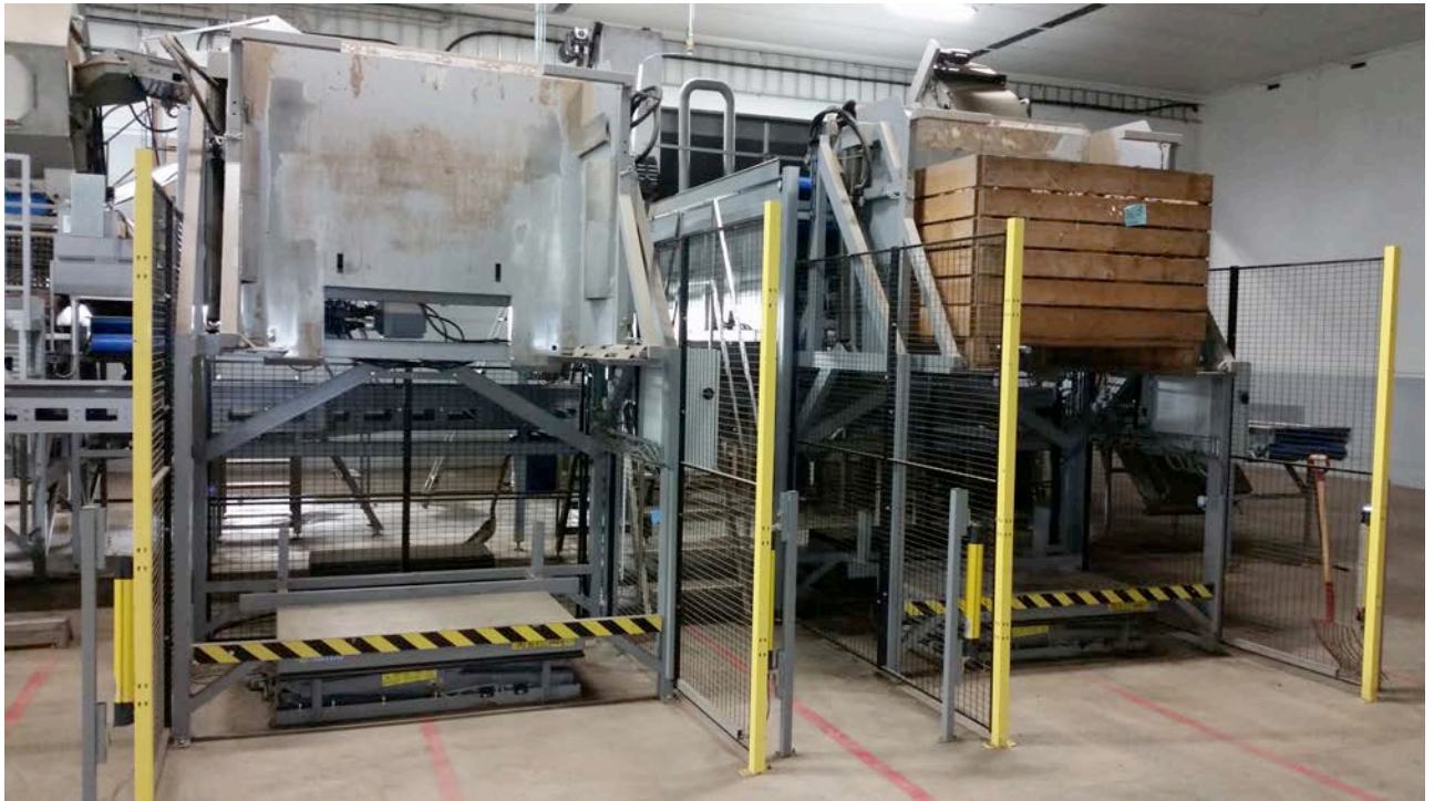
Feeding via parallel double Boxturners.
