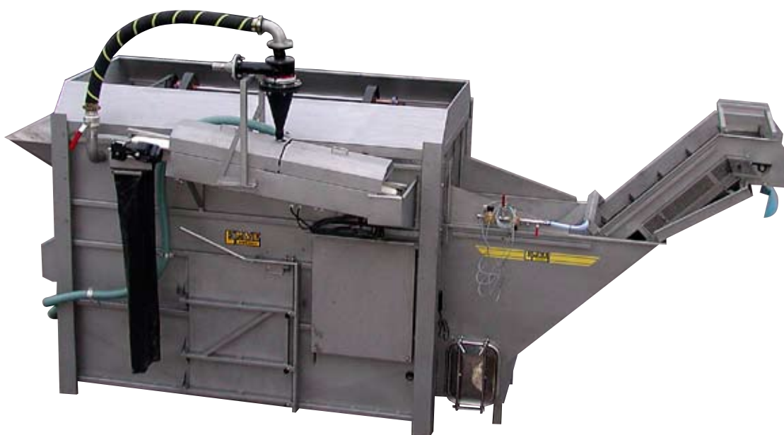
Washer with Akva-sep water recycling
